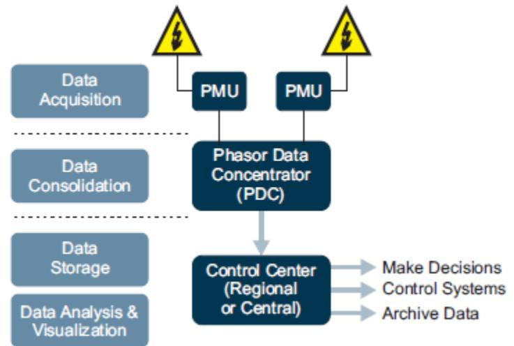
After collecting and time stamping phasor data, the PMUs send the data to a phasor data consolidator (PDC). PDCs have servers that receive data from multiple PMUs and consolidate it before transmitting it to a regional or central grid control center. PMUs collect and send a massive amount of data to PDCs. Sophisticated telecommunications technologies such as fiber optic cables and satellites are an integral part of the synchrophasor networks. For example, two
