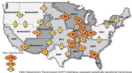
High Opportunity Transmission (HOT) interfaces represent potentially beneficial transmission capacity expansion between regions. Transmission projects that align with these HOT interfaces could serve as a starting point for accelerated transmission expansion studies.
